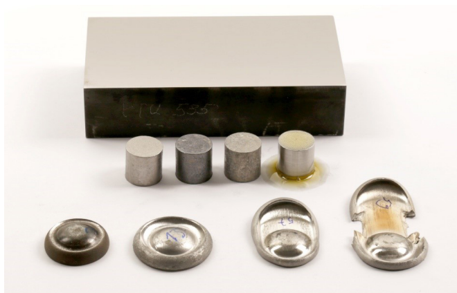
[1] Tribometer samples and tools of the Sliding Compression Test
