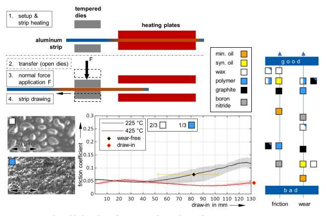
[1] Testing procedure of the heated strip drawing test with exemplary results
