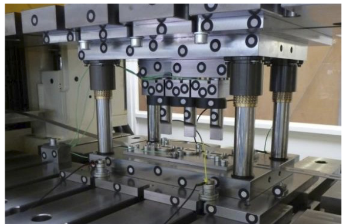
[1] Tool with reference points used for optical vibration analysis
