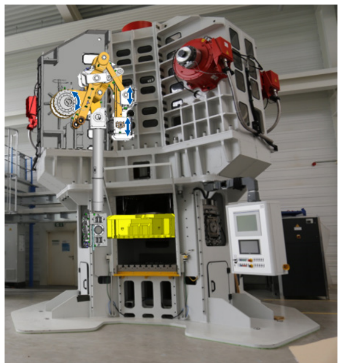
[1] 160t version of the 3D Servo Press with schematic representation of the gearbox
