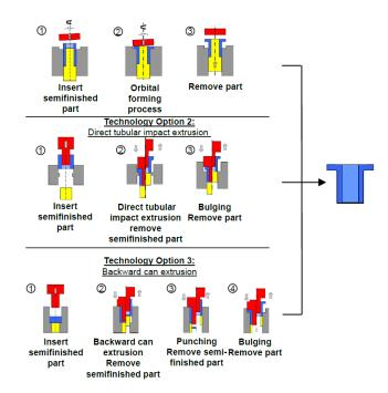
[1] Process stages of the three technology variants on the 3D servo press [GROCHE, P, et al. Rechnet sich Flexibilität in der Umformtechnik. Does Flexibility Pay Off, 2010]
