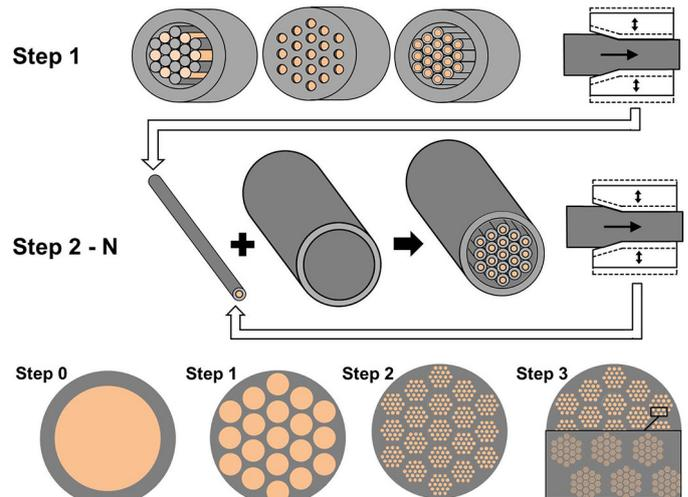
[1] Concept of forming metal-matrix-composite for magnetic materials
