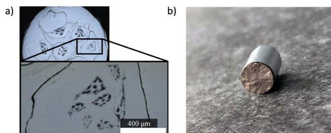
[2] a) MMC structure made of NdFeB (dark) and 1.4301 stainless steel (light) processed by rotary swaging and b) NdFeB magnet encased with stainless steel foil
