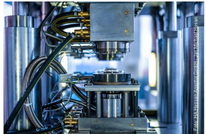
Figure 2: Side view of the four-stage forming tool including the cooling, heating and thermocouple connections
