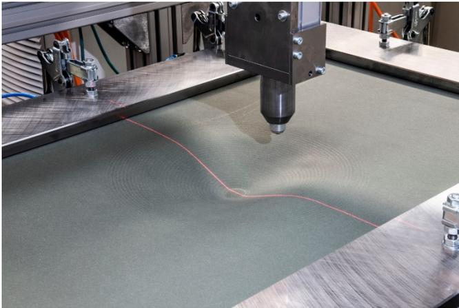
Figure 2: 3-Axis Gantry System with Vulcanized Fiber Cone during Geometry Determination by Means of Line Laser
