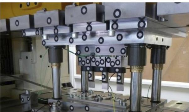
Figure 1: Tool with markers for optical measurements.
