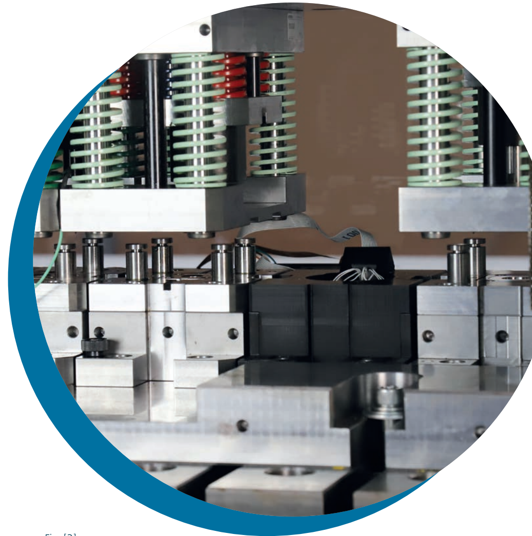
Fig. [3] Photometric stereo scanning module lined in progressive die tool
