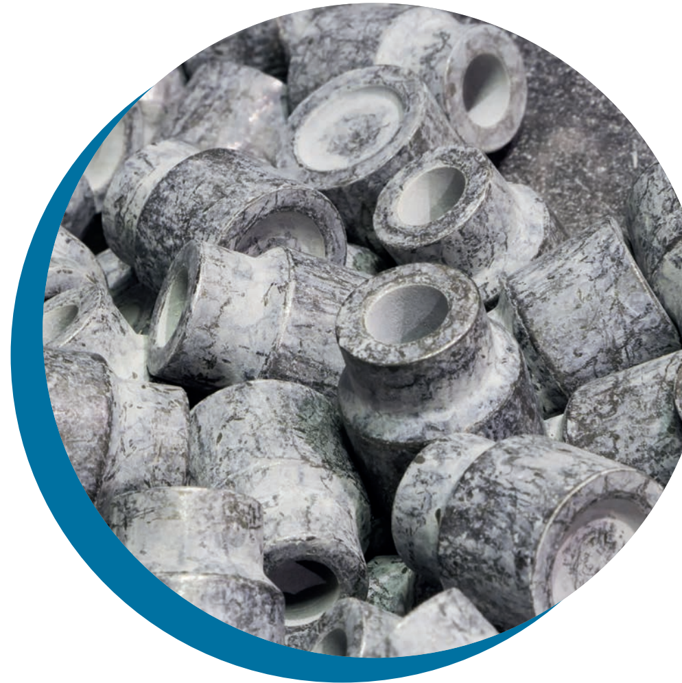
Fig. [3] Workpieces in cold forging coated with ZnPh and soap
