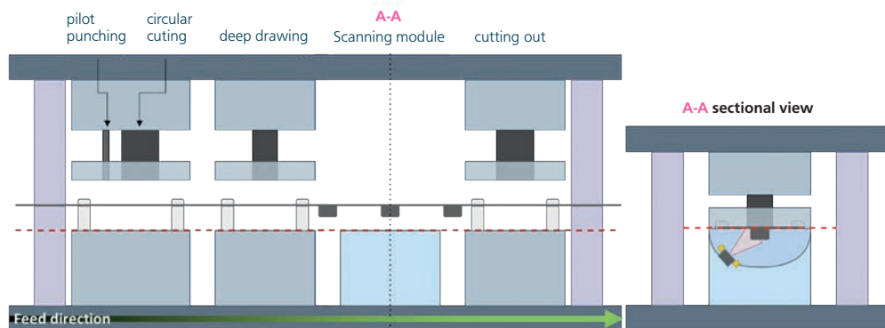
Fig. [2] Test setup in the endurance test with pilot punching, (1) circular cutting, (2) deep drawing, scanning module and (3) cutting out
