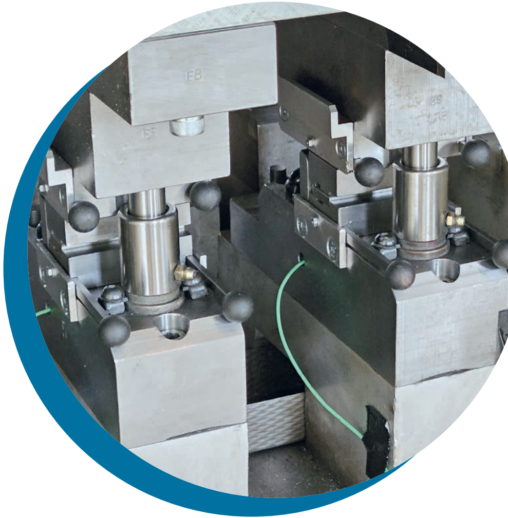
Fig. [3] Sensor retrofit of a blanking press for monitoring force and acceleration
