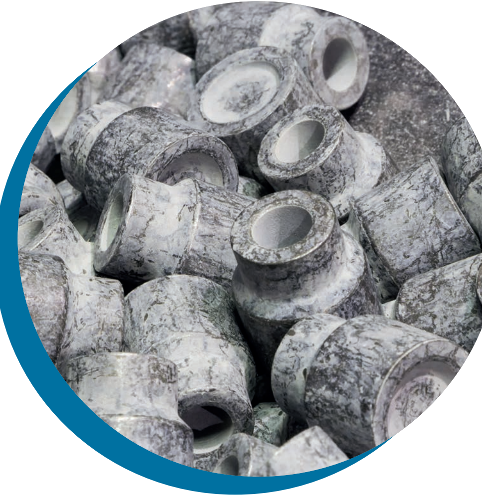
Fig. [3] Workpieces in cold forging coated with ZnPh and soap
