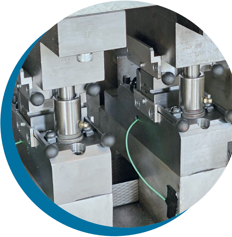
Fig. [3] Sensor retrofit of a blanking press for monitoring force and acceleration
