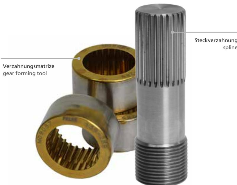
*Wear investigation and prediction in gear forming processes with oscillating ram movement*
